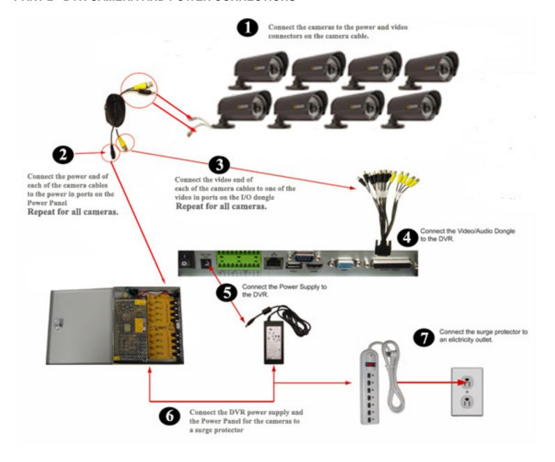
Please note that it is STRONGLY recommended to use a surge protector that is UL-1449 rated. Look for a clamping voltage of 330 or lower, a Joule rating of at least 400 and a response time of 10 nanoseconds or less.
